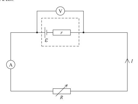
(a) As the resistance *R* of the variable resistor is varied, values of the current *I* in the circuit and the terminal potential difference *V* across the cell are recorded.
